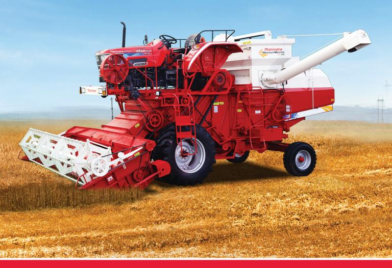
Mahindra HarvestMaster H12 2WD is a multi-crop harvester designed and developed by Mahindra as a perfect match for the Mahindra Arjun Novo series of tractors. The machine delivers superior performance in both dry and semi-wet conditions.
