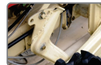
Wheel Height Adjustment for Different Soil Depth
