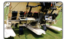
Seedling plantation depth adjustment according to height of nursery
