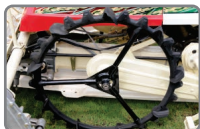
Rubber Long Life Lugged Wheel for Better traction While Transplanting
