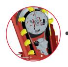
Mechanical Vibrator (Belt Vibrator)
